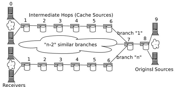
Fig. 1. Example topology with requesters on the left, original sources on the right, and potential caches along the path.
