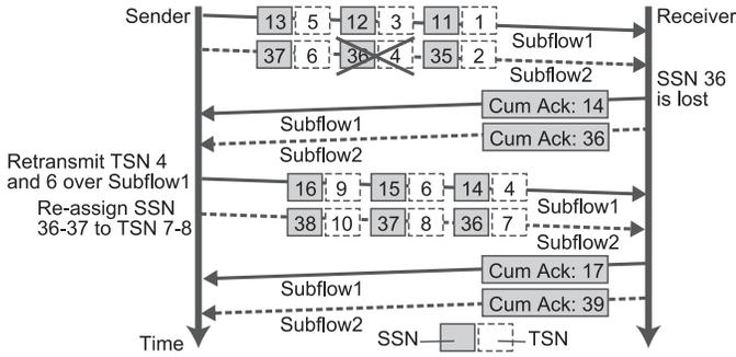
Fig. 3. One RPP connection sending over two subflows, showing transport sequence numbers and subflow sequence numbers.
