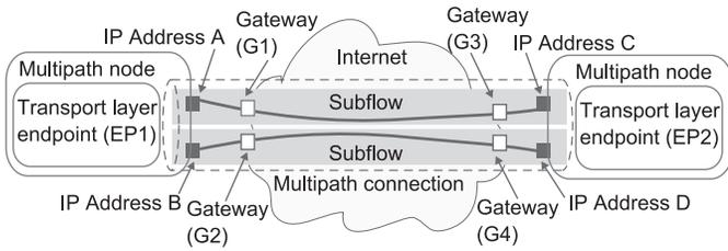
Fig. 1. One RPP connection consisting of two subflows.
